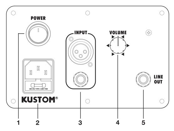
1. POWER: This switch activates AC power to the powered speaker. When the switch is illuminated, the unit is ON.
