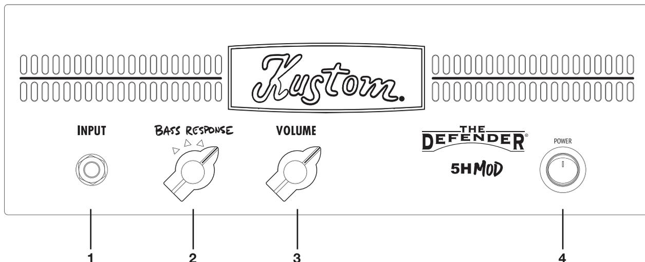
**1. Input Jack:** This is a 1/4-inch, 2-conductor input for plugging in your instrument. It is intended for guitar but will accept other instruments as well.
