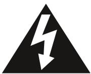
THIS SYMBOL IS INTENDED TO ALERT THE USER TO THE PRESENCE OF NON-INSULATED "DANGEROUS VOLTAGE" WITHIN THE PRODUCT'S ENCLOSURE THAT MAY BE OF SUFFICIENT MAGNITUDE TO CONSTITUTE A RISK OF ELECTRIC SHOCK TO PERSONS.
