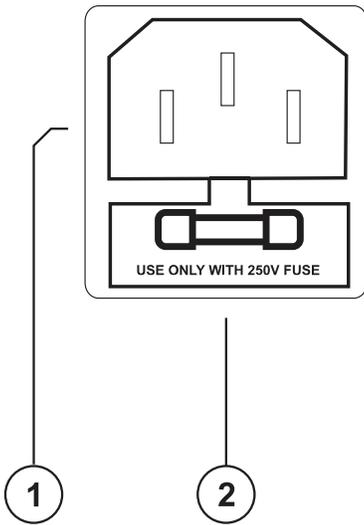
**1. AC Power Cord Receptacle:** AC power cord can be removed for easy storage and replacement if damaged. Insert the AC cord (provided) firmly into the AC receptacle. **NOTE:** Replace the AC power cord if protective jacket is damaged or ground pin is damaged or removed.
