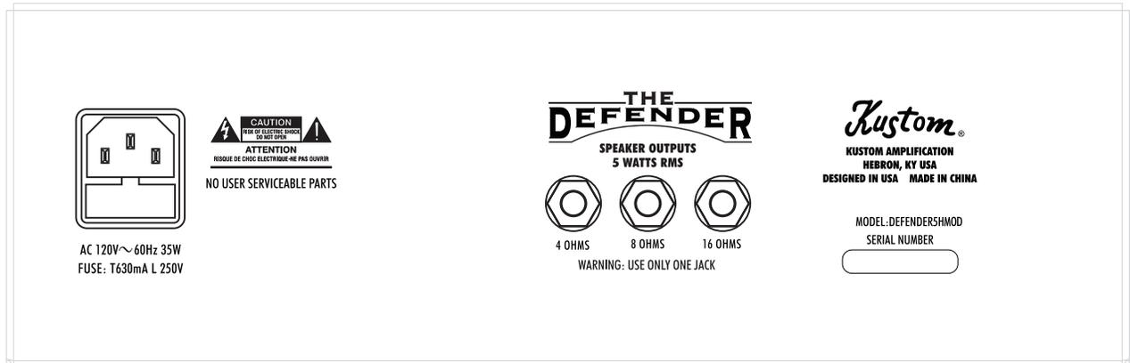
**Speaker Output:** These three ¼-inch jacks are for use with an external speaker cabinet. The Defender 5H MOD may be used with one speaker cabinet rated at 4-, 8- or 16-ohms. Be sure to connect the speaker cabinet to the correct output jack with the matching impedance.
